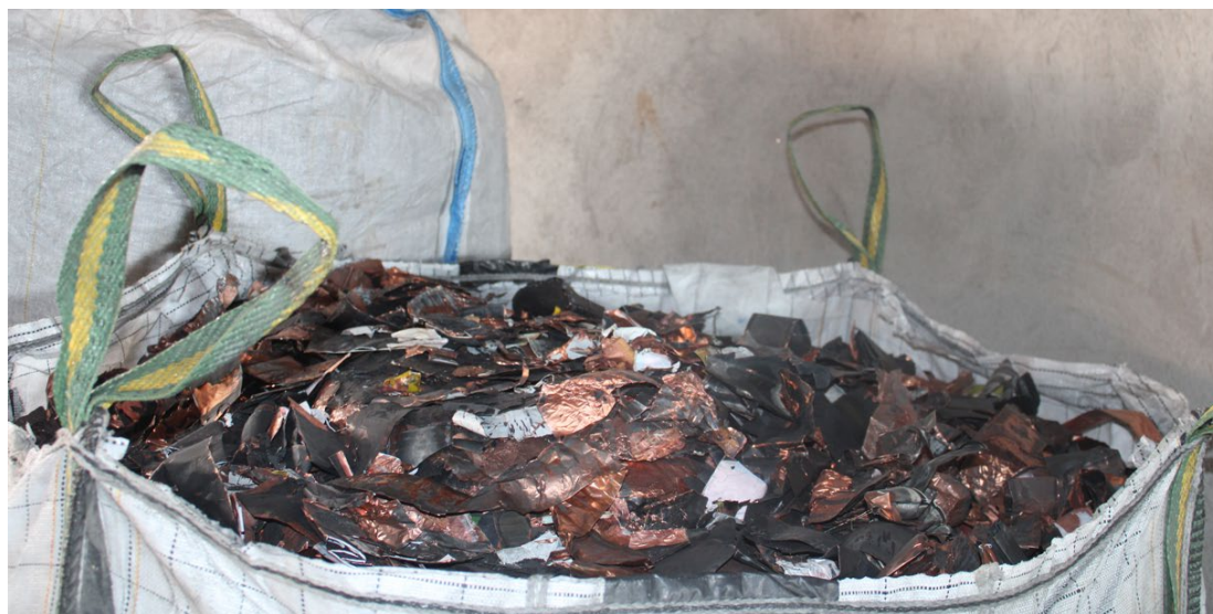
Figure 3: Electrodes (mainly graphite on copper foil) from manual LIB dismantling
